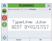
A preview of print layout confirms the correct job has been loaded and gives operators confidence that the data entered is correct prior to printing.
