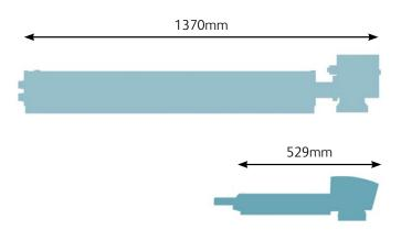
Size comparison is based on a Videojet 7610 fiber laser and 100-Watt Nd:YAG
