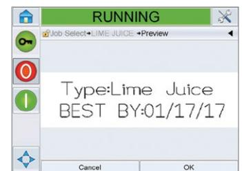
A preview of print layout confirms the correct job has been loaded and gives operators confidence that the data entered is correct prior to printing.
