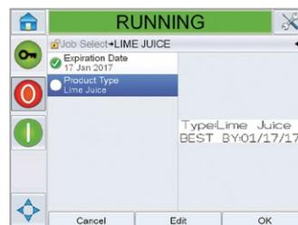
Based on pre-defined job set-up rules, only permissible fields can be edited. The print job can be loaded only after the operator has confirmed each entry.
