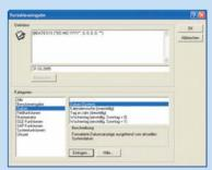
In addition to the classic **variables** such as date, counter or customized entry, Labelstar PLUS provides also other functions, e.g. link of fields or mathematic calculations.
